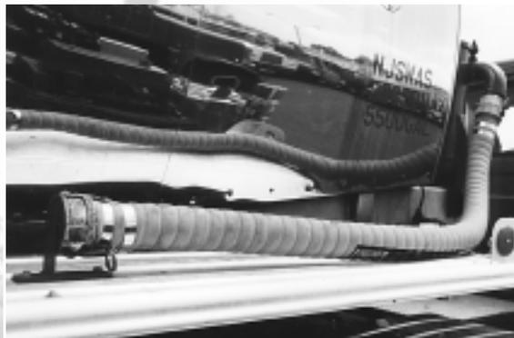
BAND-IT clamps are used on many hoses for a variety of applications.
