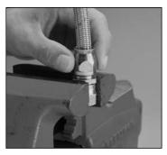
Push socket forward and handstart threading of socket to nipple.
