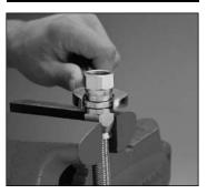
Tighten further to align corners of nipple and socket hexes if necessary.
