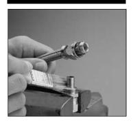
Using a SAE 20 lubricating oil, lubricate nipple and socket threads. For stainless steel fittings use Parker 702 Oil or a molybdenum type lubricant. For hose used in oxygen service lubricate using a non-oil based soap solution.
