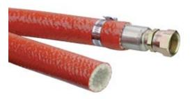
PARKER/PAGE Fire Sleeve has a coating of specially compounded silicone rubber bonded to a low density high bulk fiberglass sleeve. This unique combination offers a temporary barrier to flame penetration and provides long term mechanical and environmental protection. Applications include steel manufacturing plants, foundries, glass factories and welding/cutting shops.
