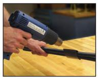
Note: EXTREME CARE MUST BE TAKEN TO AVOID EXPOSING THE HOSE ASSEMBLY TO THE DIRECT HIGH TEMPERATURES OF THE HEAT GUN WHILE INSTALLING THE HEAT SHRINK SLEEVE. LONG EXPOSURE FROM A HEAT GUN MAY ADVERSLEY AFFECT THE HOSE INNERTUBE OR ITS COVER.
