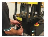
Note: EXTREME CARE MUST BE TAKEN TO AVOID KINKING THE HOSE THAT IS NOT BEING CRIMPED DURING THIS PROCESS.
