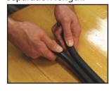
Note: It is important that the knife blade be perpendicular to the hose during this procedure so the blade cuts only the centerline of the valley (web). EXTREME CARE MUST BE TAKEN TO AVOID CUTTING THROUGH THE COVER OF THE HOSES AND THEREBY EXPOSING THE HOSE REINFORCEMENT. If this occurs, the hose assembly must be discarded.
