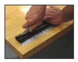
B.) To start the cut, place the blade in the center of that valley (web) drawing the knife toward you with constant pressure.
