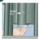
With the pusher in the full up position, lift the back half of the split die ring. Lock it in the up position by pushing the slide pin in. (The slide pin is located inside the pusher at the back.)
