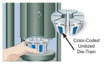
Lubricate die bowl using a premium quality lithium-base grease. Place unitized dietrain into the adapter bowl. Select die and die ring by hose size and type. See decal on crimper for proper die set.
