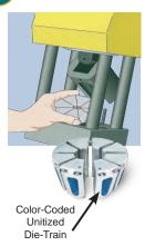
Pull pin at the top of pusher to swing it back. Place unitized die-train into base plate. See decal on crimper for proper die set. Note: Parkrimp 1 does not have a pin at the top of the pusher.
