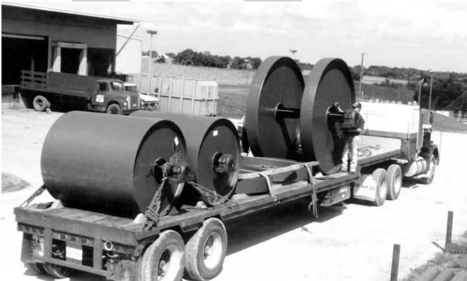
11 foot diameter deflection wheels used in a coal mine.
