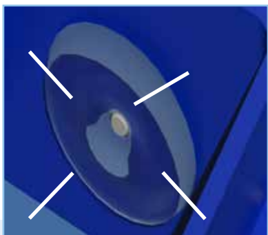
Opened radial nozzle omits airburst along the chute wall up to 24" for a tenth of a second
