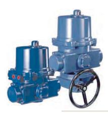
These actuators are designed to provide fail-safe positioning of valves upon loss of power. A mechanical spring set is used to position the valve in either the OPEN or CLOSED position without any external power source. A mechanical buffer is utilized at the end of the spring stroke to reduce dynamic effects. The actuator is available with or without a manual over-ride.
