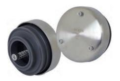
Tank Vent Valves are used for relieving pressure as the fluid level rises while filling a tank and relieving vacuum as the fluid level drops while emptying a tank.
