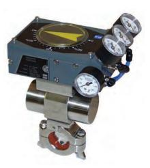
**B5102** Series Butterfly Valve with horizontal stainless steel air to open, air to close, 3-15 PSI pneumatic positioner and full gauge set.
