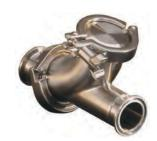
Y-ball check valves are used where full flow and low pressure drop of product during processing is required. When the flow of product stops, the PTFE ball rolls back and seats, thus preventing backflow. The two-piece body design is available in 11/2" - 3" sizes.
