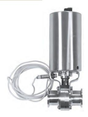
**B5101** series butterfly valve with vertical canister air to open, spring to close actuator. Normally closed, 110VAC control top
