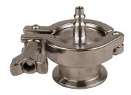
Air-blow check valves are used to clear lines of product or CIP solutions. Air connections available are 1/4" air quick coupler, 1" hose barb and 1/2" FNPT. The air-blow check valve is stocked in 1" - 4" sizes.
