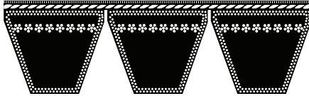
Envelope 5V, 8V Cross Section
