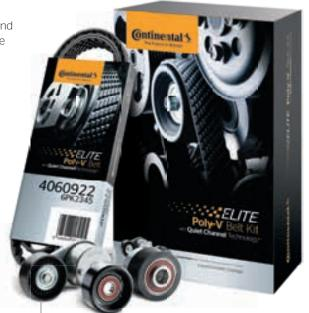
**Tech tip:** Because belts and tensioners have similar OE design life targets, it is often best practice to replace the tensioner when replacing a worn or broken belt. Doing both together will extend accessory drive life and decrease overall labor costs.
