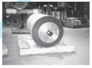
Roller assembly with a special milled slot for mounting.
