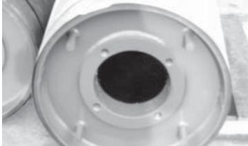
Drum pulley with speed indicator targets welded to the end discs.
