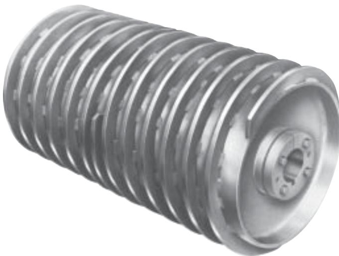
The VAN GORP® Spiral Drum Pulley is formed by a pair of vertical steel bars helically wound around a heavy-duty reinforced drum pulley (H•D•R®) and towards one another with intervals between the convolutions of each. This unique design reduces the possibility of material build-up between the belt and the pulley in applications where self-cleaning wing type pulleys cannot be used.
