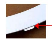
316ss tabs secure the gasket into the Cover Groove to prevent the gasket from falling out.
