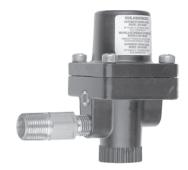
Automatically drains liquid water and oil from compressed air receivers and systems. Drain valve automatically opens and closes every time the system pressure drops approximately 10 PSI during the compressor cycle. An internal piston design, which utilizes no floats, minimizes the risks associated with drain failures.
