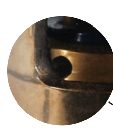
uses 3/8" rod: <30 ft lbs required to adjust
