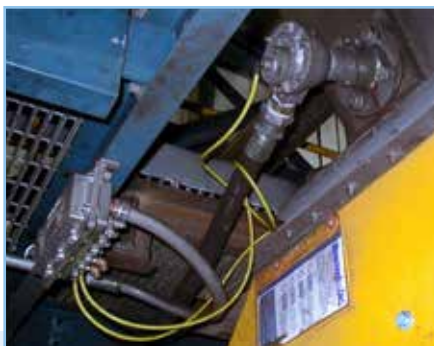
PACS is the only radial, pneumatic cleaning system specifically designed for bulk material handling and designed to not damage
