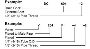
Tube sizes are determined by the number of sixteenths of an inch in the tube O.D.
