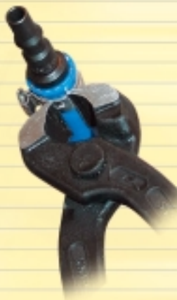
To remove a Stepless Ear Clamp, grasp the strip end with the pincer and pull it away
