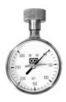
Regular pressure hand pushes LAZY hand to peak operating or surge pressure point where it remains until you manually reset it. Excellent to determine if P/T valve is leaking from failure or if leaking is caused by surge of excessive pressures. (Attach gauge to Boiler Drain Valve overnight.) LAZY hand operates over entire gauge range of 0-300psi
