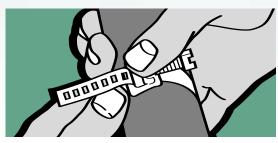
Insert band thru buckle from underneath. Pull band snug about pipe and engage serration of band on inner lug.
