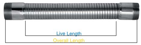
To calculate the proper length of a hose assembly you should follow these steps:
