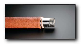
Insulating Jackets - If the corrugated hose is to convey hot media, and there is a potential for skin contact, an insulated, protective jacket is available. The jacket consists of a tubular braided fiberglass insulation, covered and impregnated with silicone rubber. The jacket is installed over the corrugated hose and metal banded in place. The jacket can also be used to insulate the corrugated assembly and either prevent ambient heat from being conveyed to the media or to reduce heat loss.
