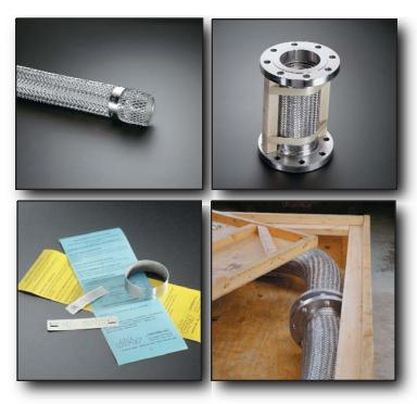
All assemblies are shipped with protectors over sealing surfaces such as threads and flange faces. Spacer bars are installed on all shorter double-flanged assemblies to prevent compression of the assembly during shipping and handling. Special packaging is available to suit customer requirements, including crating, plastic bagging, labeling, and custom fitting protectors.
