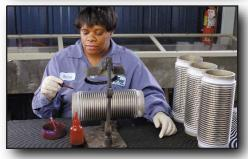
**Dye Penetrant** - Dye penetrant testing is available for both leak and for weld bead inspection, in accordance with Hose Master procedures or to customer specified standards.
