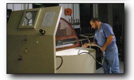
*High Pressure Gas* - Testing with air under water, at pressures of up to 2500 psi, is available for specialized applications. For a more sensitive test, the use of gases such as nitrogen or helium can be requested.
