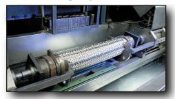
**Standard Leak Testing** - Every corrugated hose assembly is leak tested prior to shipment. Standard testing consists of pressurizing the assembly with air and then submerging the entire assembly under water. This method is reliable and sufficient for the majority of applications.
