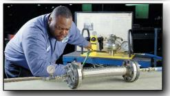
*Hydrostatic Testing* - While the standard test is designed to detect leaks, hydrostatic testing is designed to test the assembly's strength. Testing of an assembly to its full permissible test pressure can be economically and accurately accomplished by filling the assembly with liquid while concurrently evacuating all air. The assembly is then hydrostatically pressurized using high pressure pumps. The test pressure is maintained for a predetermined period of time.
