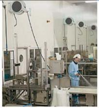
Note: Reels are primarily for manual pullout applications with lift height no more than 17ft. Otherwise, please call factory for application assistance. For hose rated up to 700 PSI.
