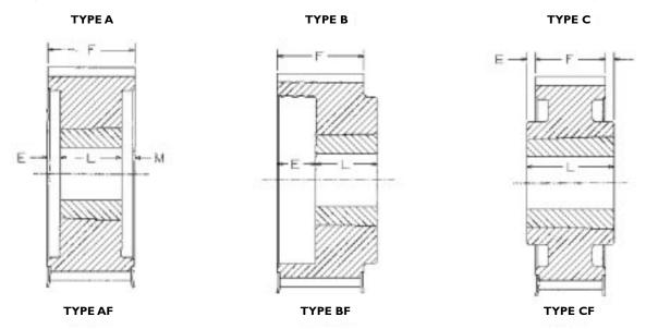
The figure following the sketch reference letter in the "Type" column indicates the construction of the sprocket (1=Solid, 2=Web, and 3=Arms), and the letter "F" indicates that the sprocket has flanges.
