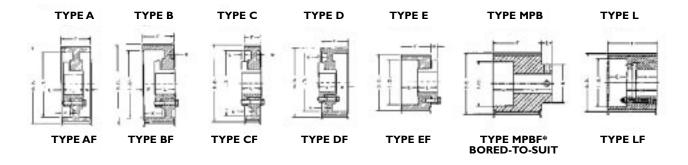
The figure following the sketch reference letter in the "Type" column indicates the construction of the sprocket (1=Solid, 2=Web, and 3=Arms), and the letter "F" indicates that the sprocket has flanges.
