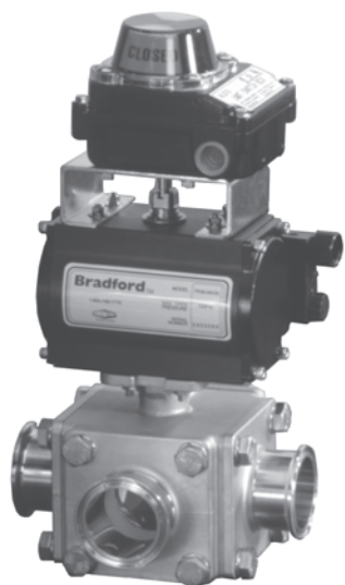
Bradford™ automated 1½" 3-way 'L'-port encapsulated sanitary ball valve with double acting actuator and NEMA 4 limit switch with two SPDT mechanical switches and NEMA 4 115 VAC solenoid pictured. BV3SVLF150CBXC
