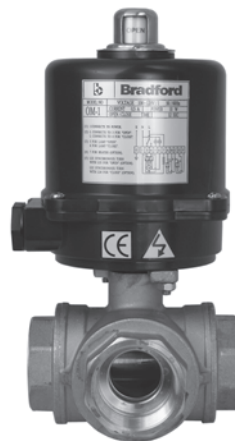
Bradford™ automated 1½" 3-way brass 'T'-port industrial ball valve with 24 volt DC NEMA 4/4x electric actuator pictured. BV3BVTR-1501-EG
