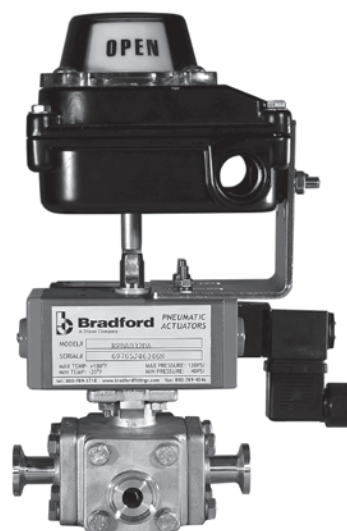
Bradford™ automated ½" 3-way 'L'-port encapsulated sanitary ball valve with double acting actuator and NEMA 4 limit switch with two SPDT mechanical switches and NEMA 4 115 VAC solenoid pictured. BV3SVLF050CBXC
