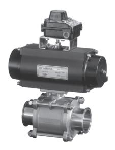
Bradford™ automated 2½" 2-way encapsulated ball valve with spring return fail close actuator and NEMA 4/4X limit switch with two SPDT mechanical switches pictured.
