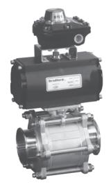
Bradford<sup>™</sup> automated 3" encapsulated ball valve with direct mount double acting, (normally open), actuator and NEMA 7 (explosion proof with 2 mechanical switches) SPDT limit switch pictured. **BV2CV-300CC-QAC**
