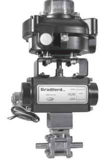
Bradford™ automated ½" encapsulated 2-way ball valve buttweld ends spring return actuator and NEMA 7 (explosion proof) SPDT limit switch with two proximity switches and NEMA 7 NAMUR mount 24VDC voltage solenoid valve pictured. **BV2CV-050BB-FPC**
