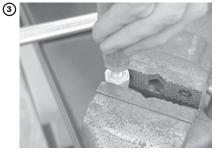
Apply lubricant sparingly to the reusable barb before inserting it into the ferrule.
