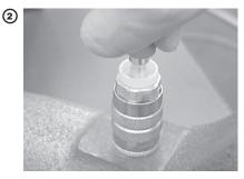
Place the end of the fitting against a flat object and grip the hose one inch from end. Push with a steady force until end of hose is covered by yellow plastic cap.
