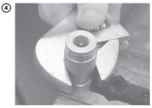
Turn the reuseable fitting into the ferrule until coupling is seated against ferrule.
