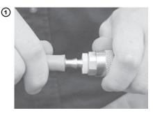
Trim hose end squarely and lubricate the Push-Loc barb and hose. Insert Push-Loc barb into hose until first barb is in the hose.
