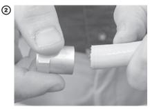
Install ferrule by slipping it onto the end of the hose and twisting it counter-clockwise.
