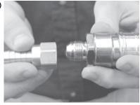
Lightly lubricate the flare on the adapter and thread it into the coupling. Hand-tighten, ensuring that the flare is seated correctly during installation.
