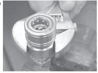
Wrench tighten the connection to the appropriate torque specification, as shown in the chart below.
