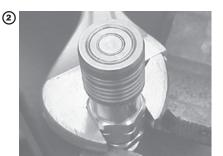
Wrench tighten the connection to the appropriate torque specification, as shown in the chart below.
