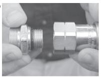
Lightly lubricate the o-ring on the adapter and thread it into the coupling. Hand-tighten, ensuring that the o-ring is not pinched during installation.
