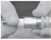
Finger tighten the connection and create a reference mark on the hex of the hose end/adapter and the coupling. This mark will help identify the number of revolutions during the next step in the procedure.
