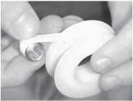
Apply 1½ to 2 wraps of PTFE tape, starting one or two threads from the lead edge, in a clockwise direction. For 316 stainless steel, be sure to use stainless grade tape.
