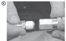
Check threads to make sure there is no obvious damage on either half and that tape is properly installed. Align male and female threaded connections and carefully begin threading the two halves together.
