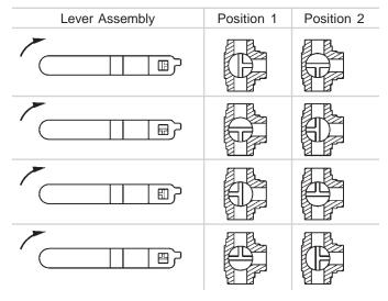
**Note:** 1/4 turn handle can be adjusted to any orientation. Notches on the valve stem reflect the three openings on the ball.
