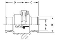
This spring check valve is machined and polished to 3A standards. It can be installed vertically or horizontally. The clamp assembly design allows quick and easy cleaning. The valve features a special design to prevent even low pressure leak through.
