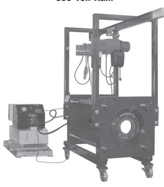
Used for swaging Holedall and Rotary fittings. This ram is capable of producing up to 354 tons of ram force for swaging. A 14" 150 lb. flange will fit through the bed plate. This ram has 36" of stroke. A 12.5 h.p., 230 volt, 60Hz, 3 phase motor is standard with remote.
