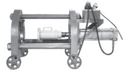
Used for swaging Holedall fittings to hose from 11/4" through 10" I.D. With optional accessories, this ram may be used for internally expanded couplings on hose from 11/4" through 6". This machine is capable of producing up to 100 tons of ram force. A 1-1/8 h.p., 115 volt, 60 cycle, single phase motor is standard with remote, (220/440 volt motors are available).
