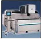
Precise shapes can be cut from any spec in Beltservice's inventory using advanced waterjet technology. A wide range of materials and dimensions can be cut with extreme precision when tolerances are critical. Exceptional edge quality is produced without inducing heat affected zones or mechanical stress. Raw materials maintain their structural integrity, and deburring is usually not required. Perforated belts can also be fashioned using our software-controlled waterjet system.
