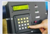
Enter the type of clamp, clamp width and type of steel. Insert clamp tail and press foot pedal. When the programmed tension is reached, cutoff and tail ejection are automatic.
