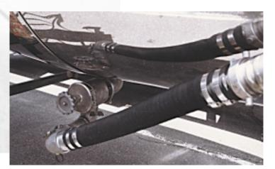
Fuel transport truck using hose for tank transfer to in-ground storage units.
