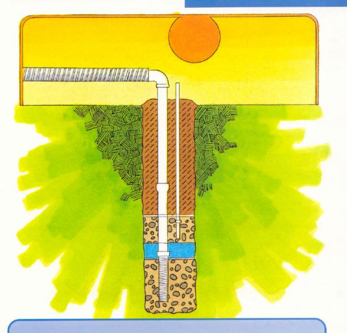
Kanaflex 101-PS PVC suction hose is specially designed for *use in methane* recovery at landfill sites. It performs well as a flexible pipeline from wellhead to main header and as a connection between rigid pipes of the same size. It is also ideal for quick emergency repairs of broken rigid lines.
